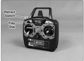
□ 1. Confirm that all four servo reversing switches in the front of the transmitter are set to *reverse*. Install batteries in the transmitter. Turn on the power and make certain the electronic trims for the surfaces (aileron, elevator, rudder) are centered.
