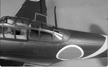
Fit the removable antenna into place through the opening in the back of the canopy – it may be a good idea to remove the antenna during transport to avoid damage.
