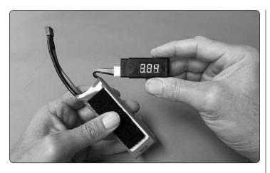
Additionally, or if you don't have a charger with a digital readout to find out how much capacity you used during a flight, use a LiPo cell checker to check individual cell voltage after each flight. The resting, non-loaded, individual cell voltage after a flight should be no less than **3.7 V/cell**.
